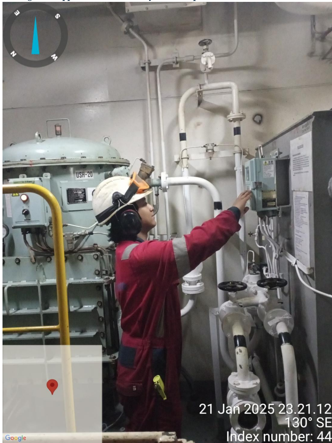
Testing the 15 ppm alarm on an Oily Water Separator
